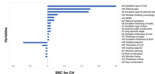
Fig. 4. Influential design variables based on a sensitivity analysis
